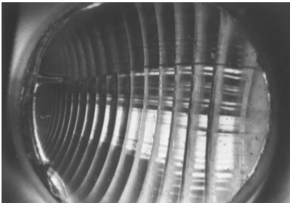
Fig. 12.18 Crack growth striations on fracture surface of \frac{1}{4} in. diam polycarbonate-resin specimen; 115 cycles to fracture. Source: Ref 12.5
