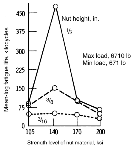
Fig. 11.29 Effect of strength level of nut material on mean-log fatigue life of threaded fastening. Source: Ref 11.36
