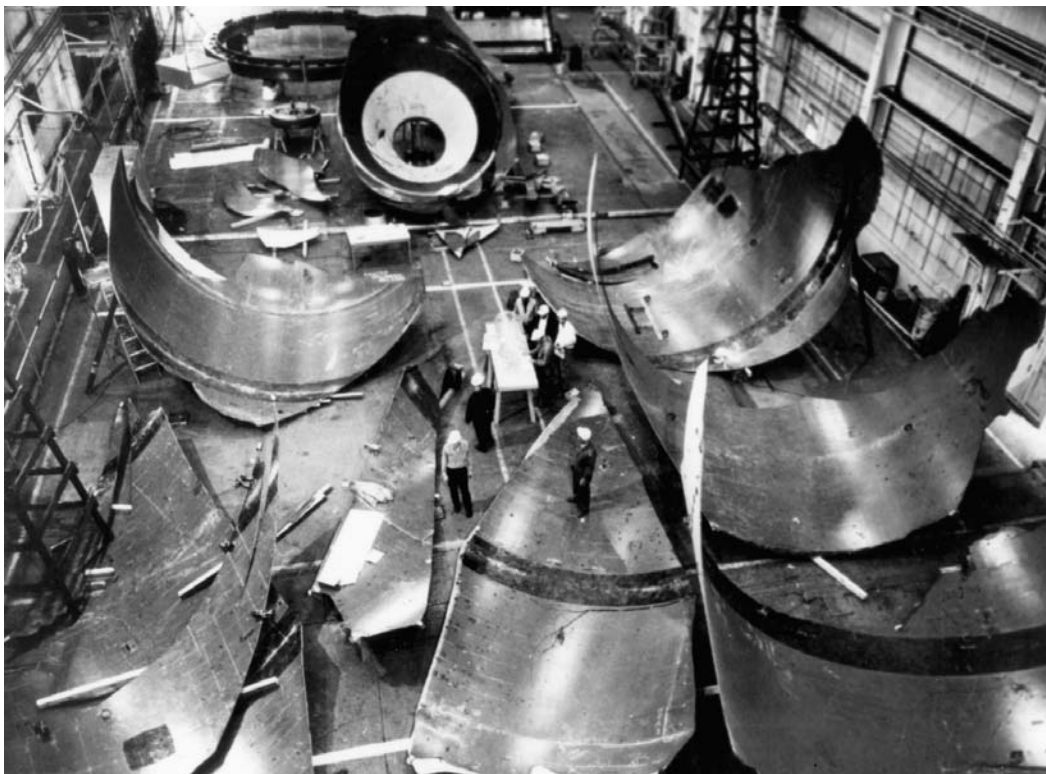
Fig. 9.3 Catastrophic brittle fracture of a 260 in. diam rocket motor case during hydrotest. Failure occurred unexpectedly at about 50% of design pressure. Note size of case compared to the 6 ft tall men.
